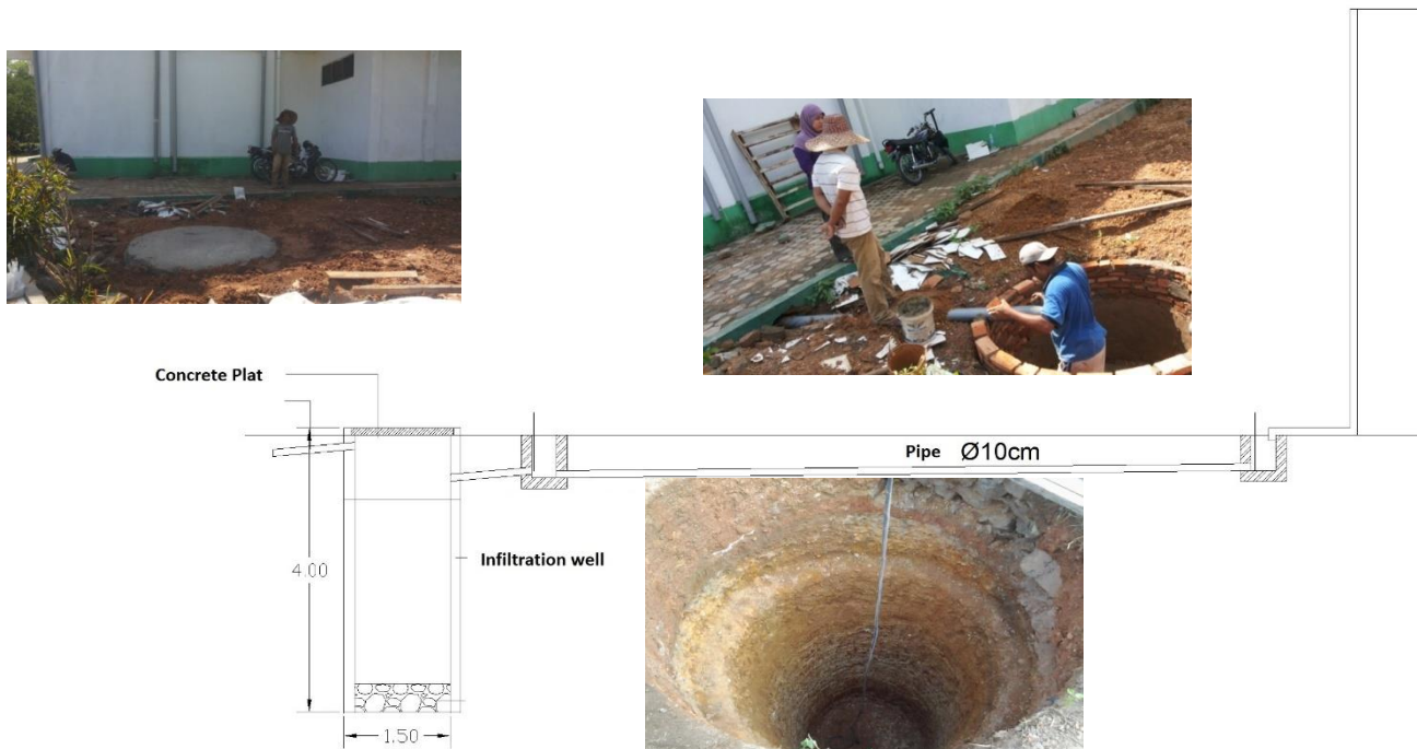
Figure 3. Infiltration well detail
