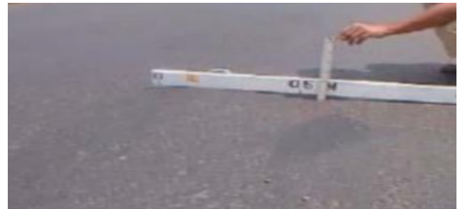
Figure 4. Example of Distortion (ruts) (Direktorat Jendral Bina Marga, 1983)
